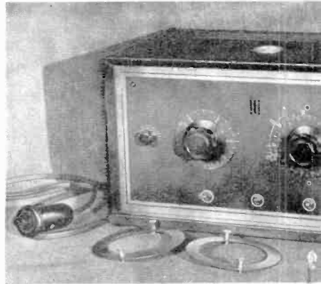
The panel view of the audiometer together with earphones of which errors are automatically corrected in different frequencies.
